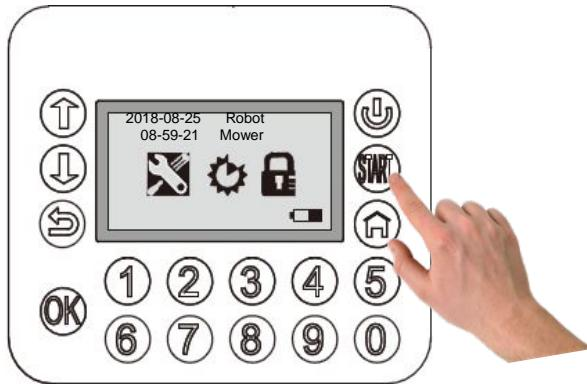
During cutting time, the battery capacity level is monitored and displayed.
