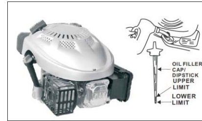
Fig. 9 CAUTION: Running the engine with a low oil level can cause engine damage. Reinstall the oil filler cap/dipstick securely.
